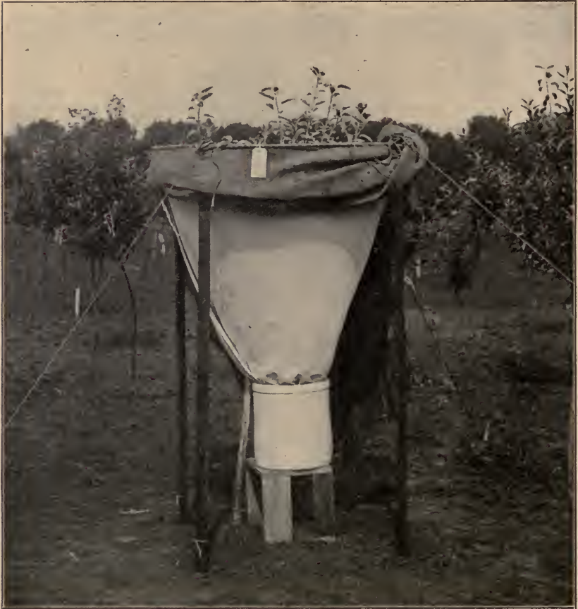
FIG. 6. Tree No. 36. Cover removed. Curtain raised to show adjustment of funnel to drip jar.
